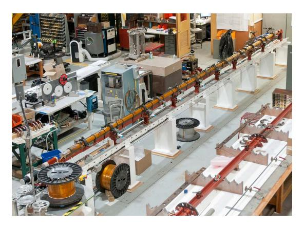
10 m coil winding machine and coil in the South Bay
